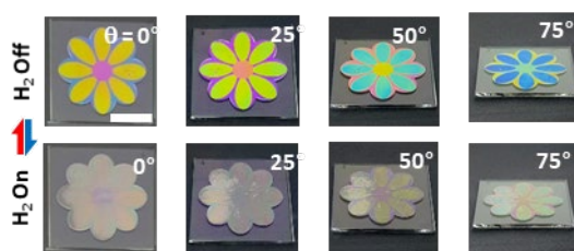
Figure 4.20: Angle-dependent color variation and foggy effect under H 2 exposure. Scale bar, 1 cm.
