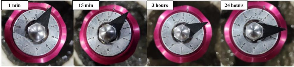
**Figure 4.10 Vane shear test results of Torvane(Exp. Scene)**
