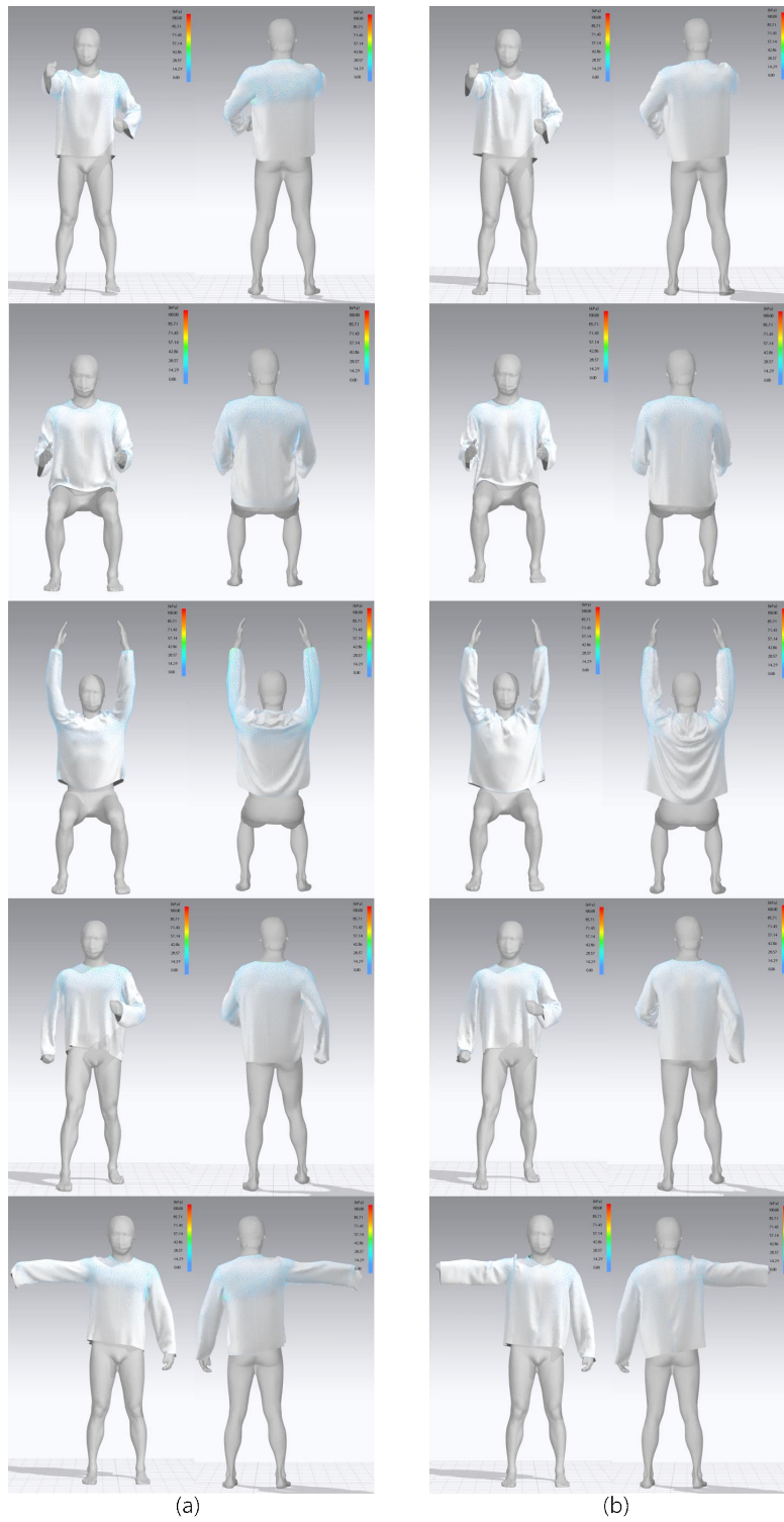
Figure 28. Averaged pattern stress map (a) Clothing pattern based on Posture 1 (b) Clothing pattern based on Posture 1~6
