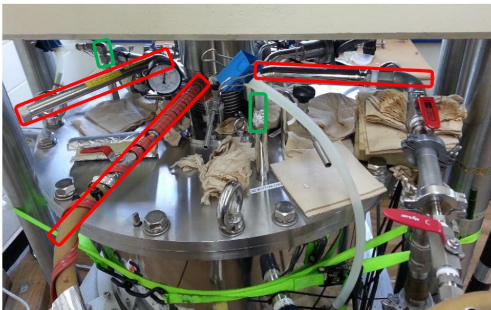
Figure A.4 A photograph displays the different transfer lines within the cubic anvil cell cryostat. The area enclosed by red boundaries denotes the liquid helium transfer lines, while the area enclosed by green boundaries signifies the liquid nitrogen transfer lines.
