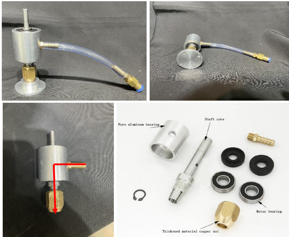
Figure 4.3 Polishing tool capable of center injection
