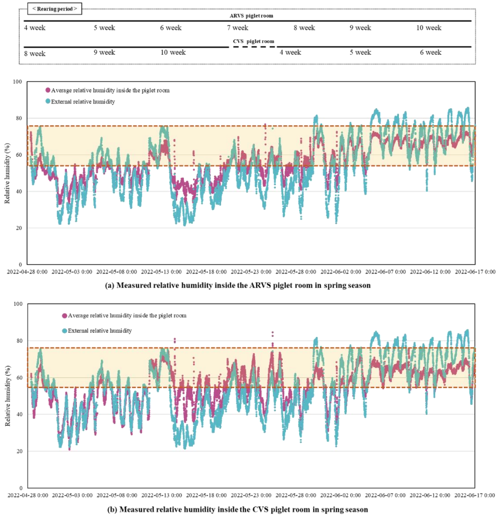
Figure 6-11 Internal and external relative humidity of ARVS piglet room and CVS piglet room in spring season during the rearing period of piglets.
