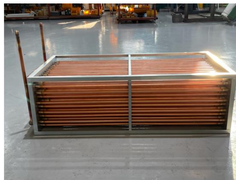
(b) Designed solar water coil for solar module
