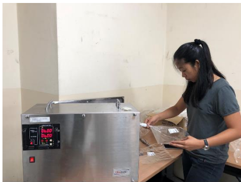
(a) Odorless air generator
