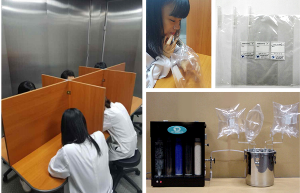
Figure 5-4. Evaluation of odour concentration using olfactometry method
