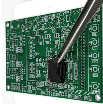
Figure 5-16. Rework tests for a Aro(0,1) D26_EV encapsulated flexible printed circuit board and b Aro(1,1) D23_EV + filler encapsulated rigid printed circuit board.
