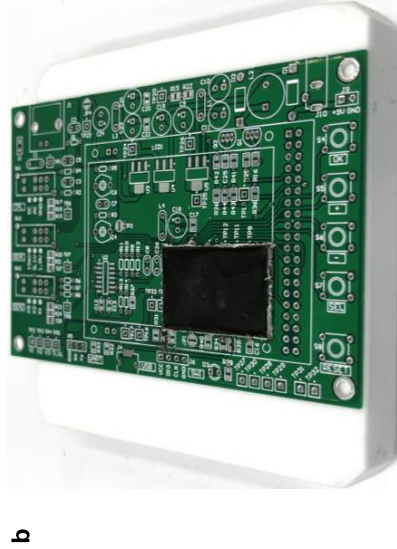
Figure 5-16. Rework tests for a Aro(0,1) D26_EV encapsulated flexible printed circuit board and b Aro(1,1) D23_EV + filler encapsulated rigid printed circuit board.
