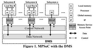
The DMS is composed of MSAPs, control network and data network. Each subsystem is connected to a specific MSAP that
