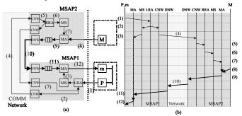
Figure 6. A data transfer example between two MSAPs
