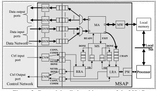
Figure 3. General detailed architecture of the MSAP
