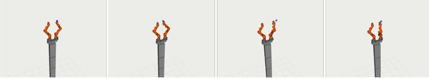
FIGURE 2.7: Snapshots of the right arm end-effector circular trajectory tracking simulation with the impedance control in (2.27)
