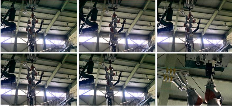
FIGURE 2.15: Snapshots of the 1mm-tolerance peg-in-hole task with the telerobotic system in mock-up environment of the nuclear power plant.
