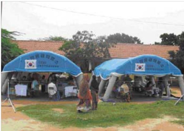
Fig. 1. Two air-inflatable tents. The left tent was a surgical unit and the right one a medical unit. These tents were inflated by two electric generators within 10 min.
