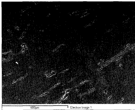
(a) Group 1 (PMMA resin and desized glass fiber complex)
