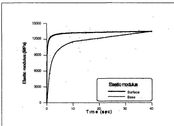
Fig. 3. Temperature dependent elastic modulus in box shape cavity.
