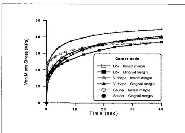
Fig. 10-3. Von Mises Stress at the corner nodes of gingival margin and incisal margin of box cavity, V. shape cavity, and saucer cavity.
