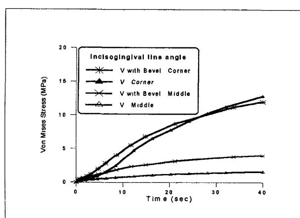
Fig. 12-3 Von Mises Stress at the nodes of incisogingival line angle of V shape cavity and V shape cavity with bevel.
