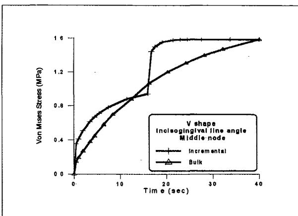
Fig. 14-3. Von Mises stress at the middle nodes of incisogingival line angle of V shape cavity.
