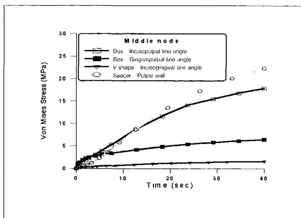
Fig. 10-2. Von Mises stress at middle nodes of axial wall of box cavity, V shape cavity, and saucer cavity.
