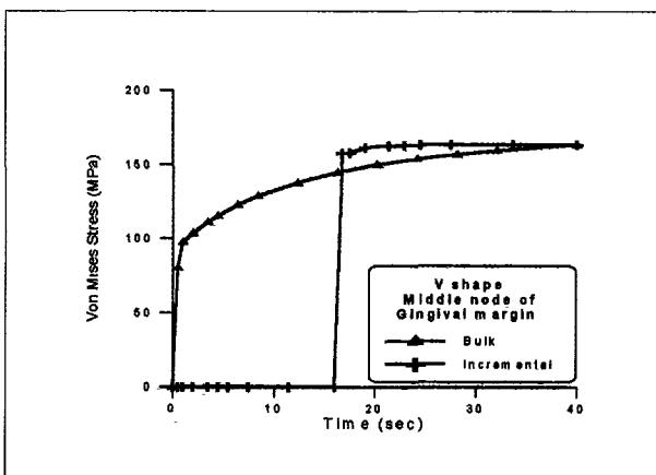
Fig. 14-1. Von Mises stress at the middle nodes of gingival margin of V shape cavity.
