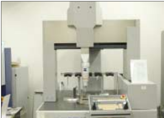
Fig. 4. Contact coordinate measuring machine (UPMC 850 Ultra, Carl Zeiss, Oberkochen, Germany).
