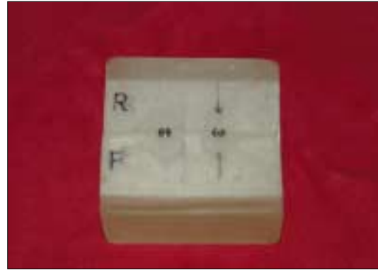
Fig. 2. Transfer jig adapted to the metal master model. The transfer jig divided into two pieces bucco-lingually was used to reduce the horizontal error occurring from mac hining tolerance of a gold cylinder.
