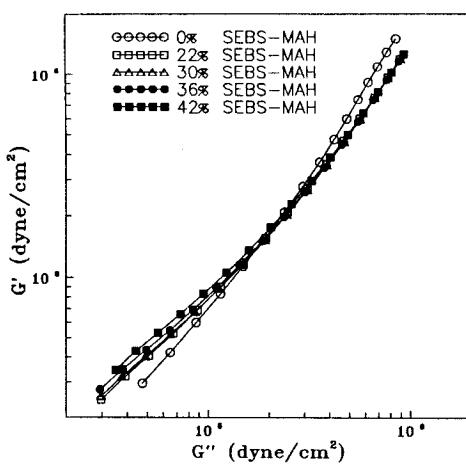
Fig. 6. Modified Cole-Cole plot of nylon/PPO/impact modifier ternary blends as a function of SEBS-MAH content in the impact modifier.
