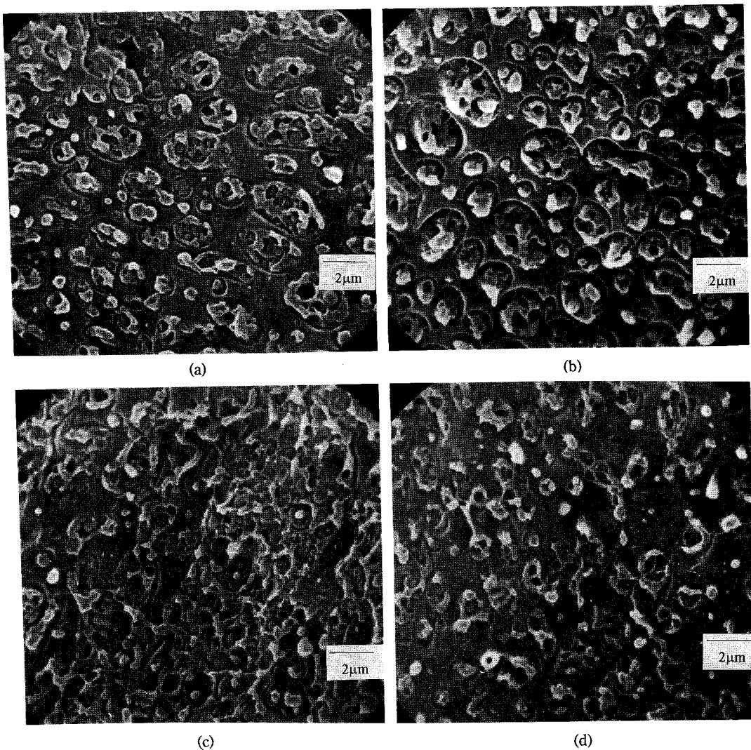
**Fig. 2.** Scanning electron micrographs of the cryogenically fractured surfaces of nylon/PPO/impact modifier ternary blends as a function of increasing amount of SEBS-MAH in the impact modifier: SEBS-MAH wt% in the impact modifier=(a) 22 wt%; (b) 30 wt%; (c) 36 wt%; (d) 42 wt%.
