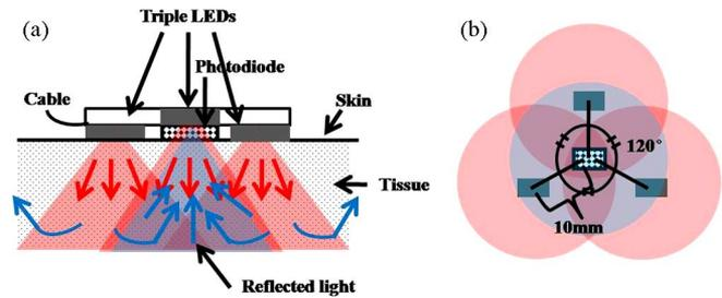
Fig. 1. Conceptual diagrams of the proposed PPG sensor with three light sources. (a) Frontal view. (b) Transverse view.
