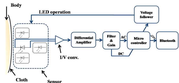
Fig. 2. Block diagram for the proposed PPG measurement system that includes an adaptive light intensity control function using dc components.
