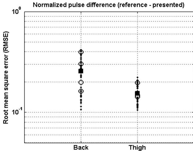
Fig. 4. RMS error for normalized pulse difference between PPG signals measured using reference and presented method. (x) Ten 6 s segments and (o) total 1-min data for each subject and (■) mean of all segment showed very low level of rms error.
