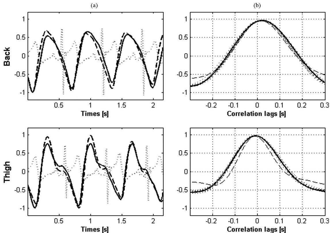
Fig. 5. (a) Example waveform of (dashed line) normalized reference, (solid line) proposed PPG, and (dotted line) ECG. (b) Cross correlation coefficients with respect to correlation lag for (dotted line) each segments, (dashed line) mean of all segment, and (solid line) total 1-min data.
