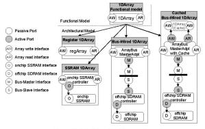
Figure 2. A CATtree for 1D array channels.
