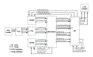
Figure 4. System function model of the H.264 decoder.
