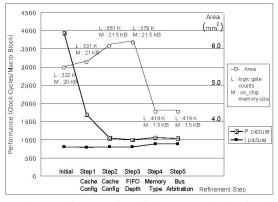
Figure 5. Performance and area of the H.264 VGA decoder after each refinement step.
