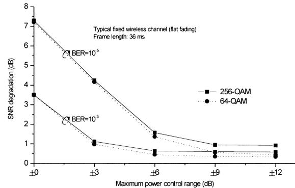
**Fig. 5** Performance degradation of proposed QAM transceiver versus power control range.
