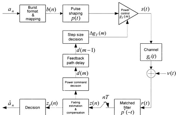
**Fig. 1** Block diagram of a baseband equivalent QAM transceiver with Tx power control.
