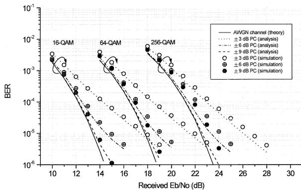
**Fig. 9** BER performance of the proposed QAM transceiver in a typical fixed wireless channel with flat fading.
