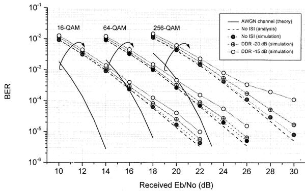
**Fig. 8** BER performance without power control in a typical fixed wireless channel.
