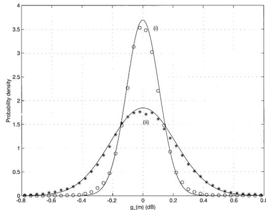
**Fig. 4** Distribution of  $g_o(m)$  in a typical fixed wireless channel: (i) solid line: log-normal distribution ( $\sigma = 0.108$  dB), symbol ( $\circ$ ): distribution of  $g_o(m)$  ( $f_d T_F = 0.0108$ ), (ii) solid line: log-normal distribution ( $\sigma = 0.216$  dB), symbol ( $*$ ): distribution of  $g_o(m)$  ( $f_d T_F = 0.0216$ ).
