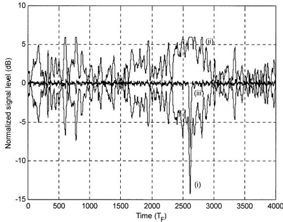
**Fig. 2** Simulated waveform of power controlled signals of QAM transceivers in a typical fixed wireless channel: (i) Channel gain, (ii) Power controlled Tx signal, (iii) Rx gain after power control.
