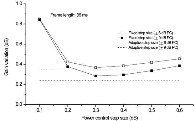
Fig. 6 Gain variation of 256-QAM signal power after the Tx power control.
