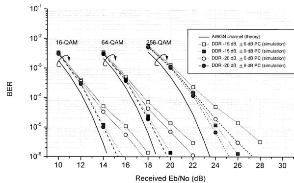
**Fig. 10** BER performance of the proposed QAM transceiver in a typical fixed wireless channel with frequency selective fading.
