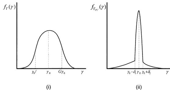
**Fig. 3** SNR distribution of the received signal in a fixed wireless channel: (i) Without Tx power control, (ii) With Tx power control.
