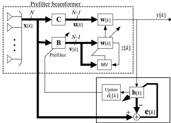
Fig. 1 Block diagram of the proposed beamformer.
