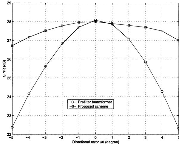
Fig. 2 SINR performance due to directional error.
