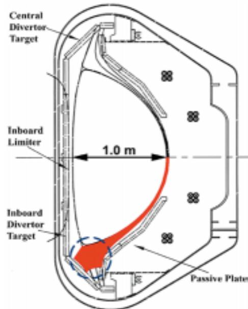
Fig. 1. Calculated domain (red-colored area) in the edge region of the KSTAR tokamak. Recycling neutral transport is considered in the dashed circle of this domain.
