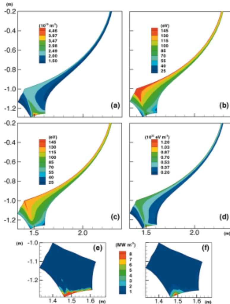
Fig. 2. Numerical images of (a) plasma density, (b) ion temperature, (c) electron temperature, (d) total pressure, (e) ion energy loss rate by charge exchange with neutrals, and (f) ion energy gain rate by electron impact ionization of neutrals.
