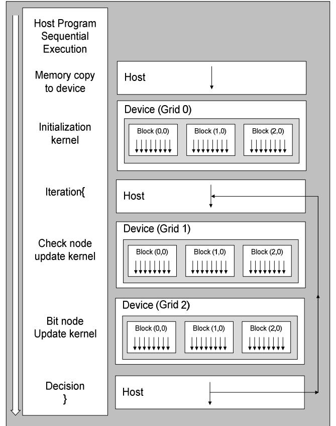
Figure 2. Devised heterogeneous programming model for SPA and MSA decoding
