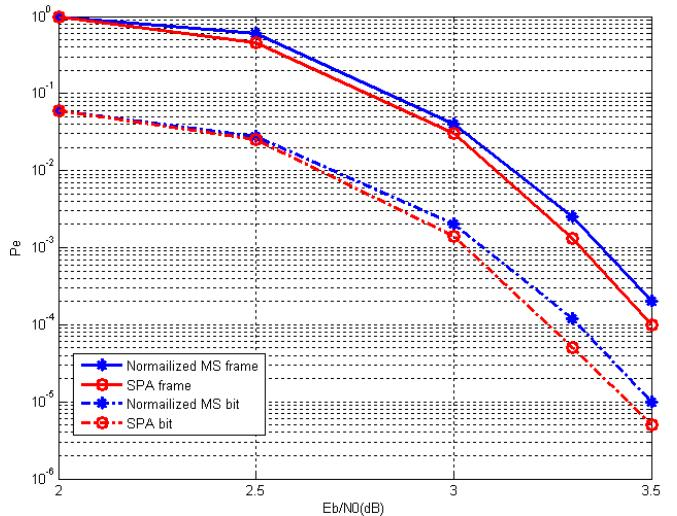
Figure 4. Error performance of the (1057, 813) PG-LDPC code
