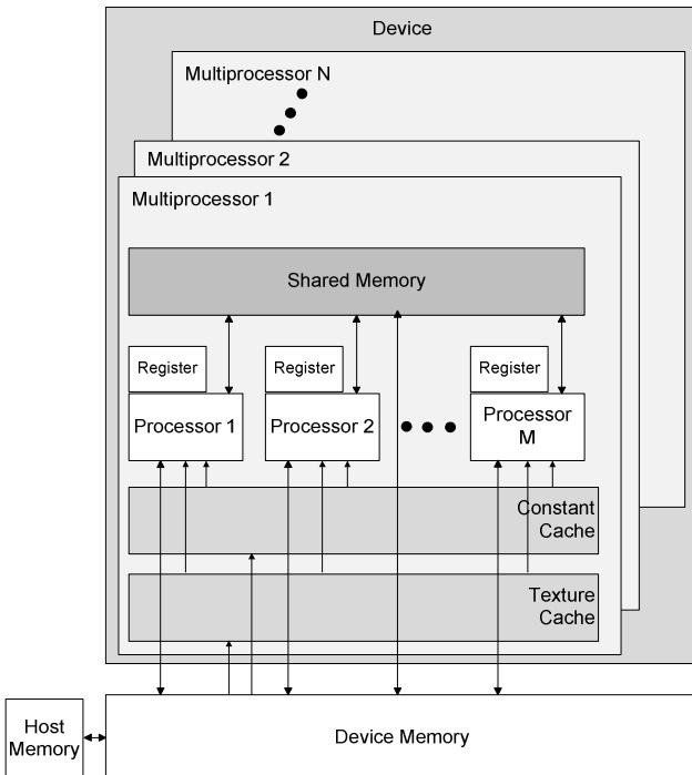
Figure 1. Nvidia GPU architecture [8]
