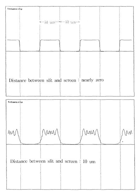
Fig. 3 DIFFRACTION PATTERN BEHIND SCREENED WINDOW 10 $\mu$ m Away (slit/space = 10/10  $\mu$ m)
