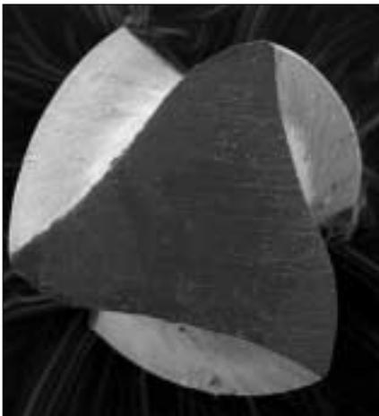
**Figure 7.** Cross-sectional electronic microscopic photograph of Hero Shaper®.
