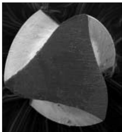
**Figure 7.** Cross-sectional electronic microscopic photograph of Hero Shaper<sup>®</sup>.
