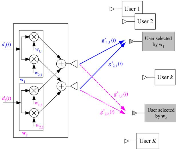
Fig. 1: The proposed MUDAM scheme applied to a (2x1) MISO system
