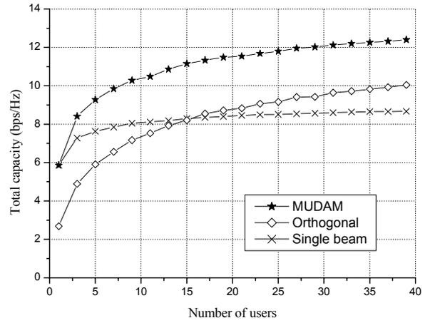
Fig. 3 The capacity in Rayleigh fading channel (SNR =20dB)
