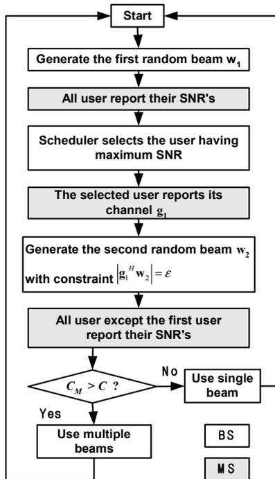
Fig. 2: The procedure of (2x1) MUDAM scheme
