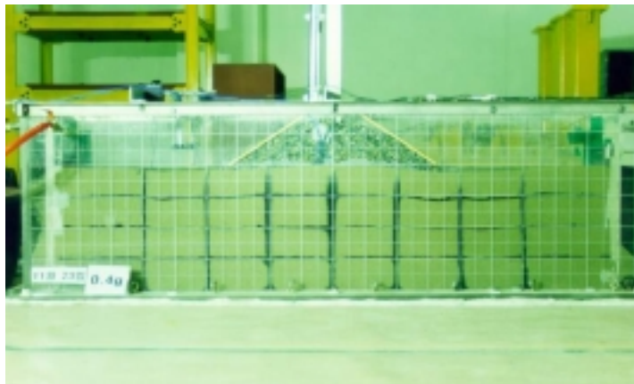
Photo 1. Deformed embankment of case 11 after 0.4g excitation
