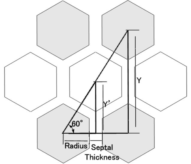
Fig. 2. Schematic of the hole pattern on the collimator. Two kinds of hole patterns were interweaved in order, and holes were formed at distances calculated using the similarity of triangles.
