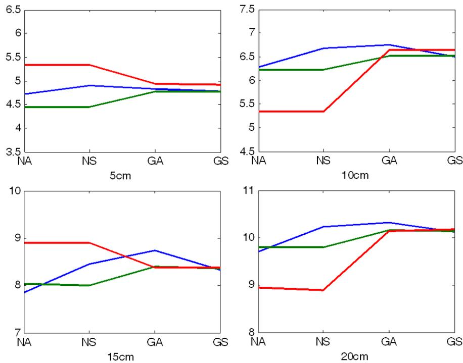
Fig. 8. Spatial resolutions of various pixel sizes and calculation methods. Blue, green, and red lines represent pixel sizes of 0.445, 0.89, and 1.78 mm, respectively. NA, NS, GA, and GS are the averaged FWHMs of each profile and the FWHM of the summed profile, which are calculated by using the NEMA method and the Gaussian fitting method, respectively.
