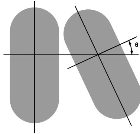
Fig. 6. Effect of rotation on the calculation of the spatial resolution. A line profile rotated by an angle  $\theta$  is miscalculated by a factor of  $1/\cos(\theta)$ .
