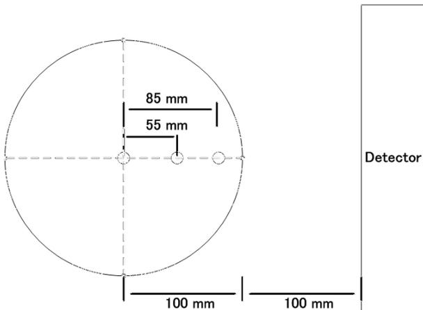
Fig. 5. Schematic of measurements for the sensitivity. A point source was placed at the center, 5.5 cm and 8.5 cm to the detector.
