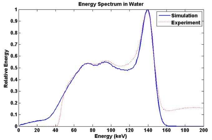
Fig. 4. Energy spectrum of a Tc-99m point source placed in a water phantom. The blue solid and the red dotted lines show the simulated and the experimental energy spectra, respectively.
