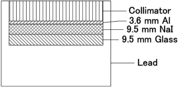
Fig. 1. Schematic of the Trionix TRIAD XLT9 triple-head SPECT detector.
