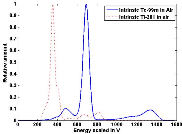
Fig. 3. Intrinsic resolutions from point sources of Tc-99m and Tl-201 without an additional phantom. The scale of the  $x$ -axis is not keV. Real energy should be restored by an interpolation of the known sources.
