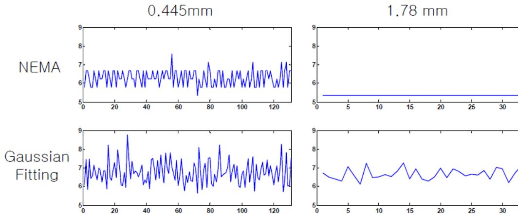
Fig. 7. Spatial resolutions at 10 cm calculated by using the NEMA (upper rows) and the Gaussian Fitting (lower rows) methods with two pixel sizes, 0.445 mm (left columns) and 1.78 mm (right columns).
