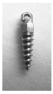
**Figure 1.** The orthodontic mini-implant used in this study (2005H, ORTHOplant, BioMaterials Korea, Seoul, Korea; self-drilling type, conical shape with 2.0-mm upper diameter, 5-mm length).
