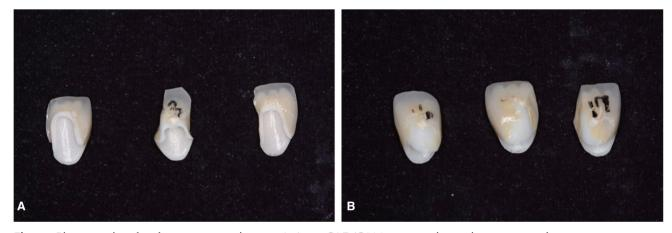
Fig. 5. Photographs after fracture strength tests. A: Lava CAD/CAM crowns showed crown core fracture pattern, B: Digident CAD/CAM crowns showed interfacial fracture pattern of core and veneering porcelain.
