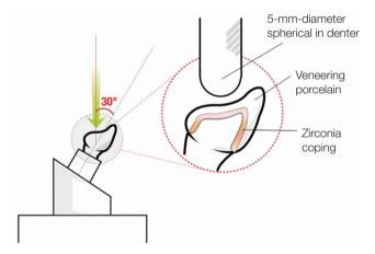
**Fig. 2.** Schematic view of the fracture strength determination procedure with CAD/CAM zirconia crowns. The direction of the load applied was 30°, and the loading points were consistently maintained by repositioning the metal die.
