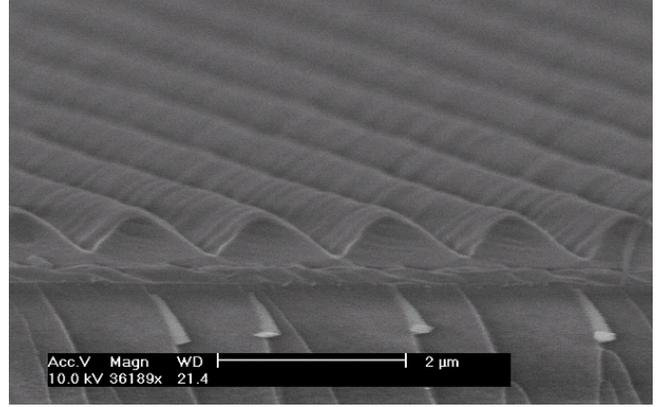
Fig. 2. SEM image of SRG on azo-dye copolymer ( $1.3\mu\text{m}$  wide, 400nm deep).
