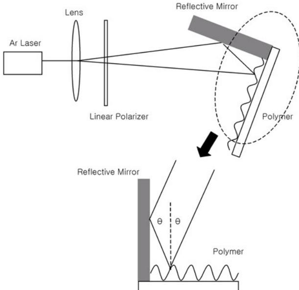
Fig. 1. Schematic view of optical setup for SRG formation. Laser beam is linearly polarized to  $+45^\circ$ . The reflected beam by mirror has  $-45^\circ$  polarization axis. Two orthogonal beams interfere on the surface of the polymer to form the groove structure. The period of grating pattern depends on the combination angle  $\theta$ .
