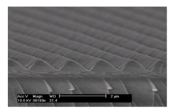
Fig. 2. SEM image of SRG on azo-dye copolymer (1.3 $\mu$ m wide, 400nm deep).
