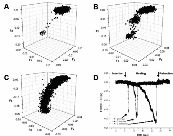
**Fig. 4** Raw data of distribution of insertion force in three-axes during epidural insertion using a type I probe (ten shanks, 100- $\mu$ m spacing) into the brain at 2 mm/sec (A), 0.5 mm/sec (B), and 0.125 mm/sec (C). (D) Z-axis components of the insertion force at each speed. Z-axis is the direction of insertion.
