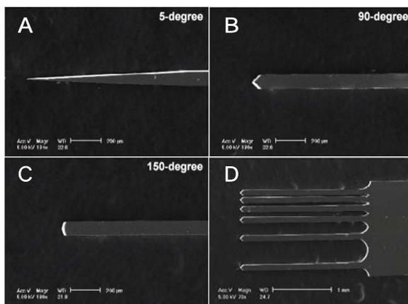
**Fig. 1** Scanning electron micrographs of the tips of fabricated silicon probes with different sharpness(A: 5degree-sharp probe, B:90degree-medium probe and C:150degree-blunt probe) and multishank array with various intershank spacing(D)
