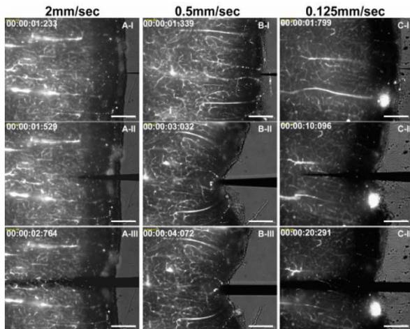
**Fig. 3** Time-lapse images of the surface deformation and haemorrhaging in the cortical area during insertion of a sharp probe with a tip angle of 5 degrees. These images were obtained during probe insertion at 2 mm/sec (left panels), 0.5 mm/sec (middle panels), and 0.125 mm/sec (right panels). Scale bars are 200  $\mu$ m.
