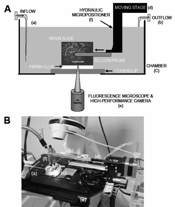
**Fig. 2** The schematic of the *in vitro* insertion setup(A). Photograph of the setup mounted on the microscope(B).
