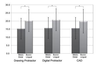
**Fig. 7.** The paired t-test results for the convergence angles measured between mesio-distally and bucco-lingually. Means and standard deviation (SD) of the abutment convergence angles are shown according to the measuring methods. Data are expressed as the mean  $\pm$  SD (n = 216). \* *P*<.05.
