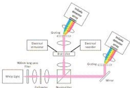
Fig. 1. Schematic design of the custom-built high-speed NIR spectrometer
